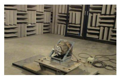
*Fig 5.0* Experimental set-up for existed fan to measure noise inside a semi anechoic chamber
